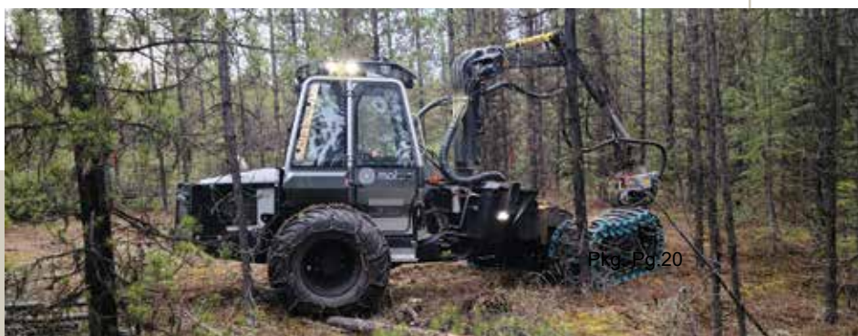
A specialized machine known as the Malwa Combi, which combines a harvester and forwarder in one Photo Credit: Mac Anderson
