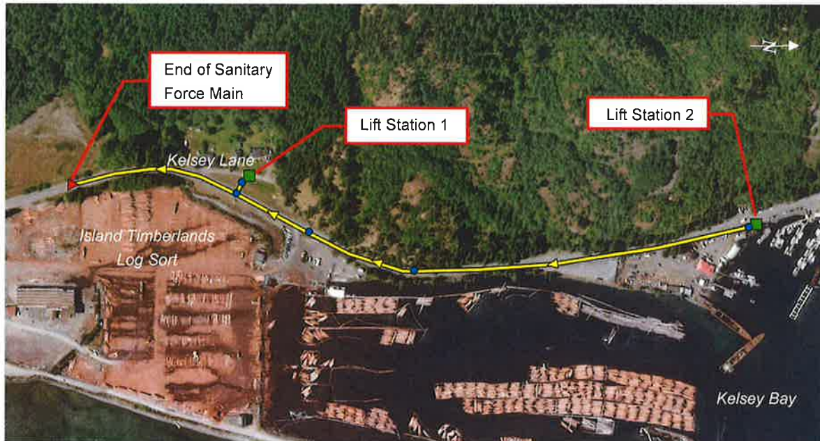
Figure 6: Existing Sanitary Force Main System
