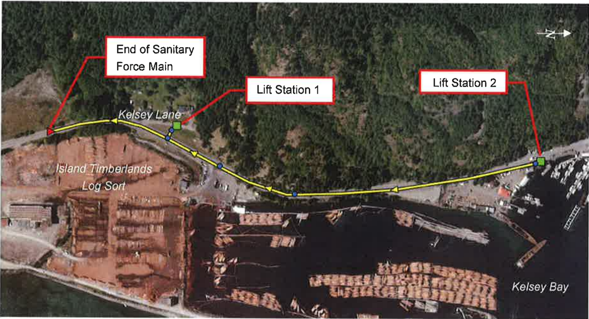
Figure 6: Existing Sanitary Force Main System
